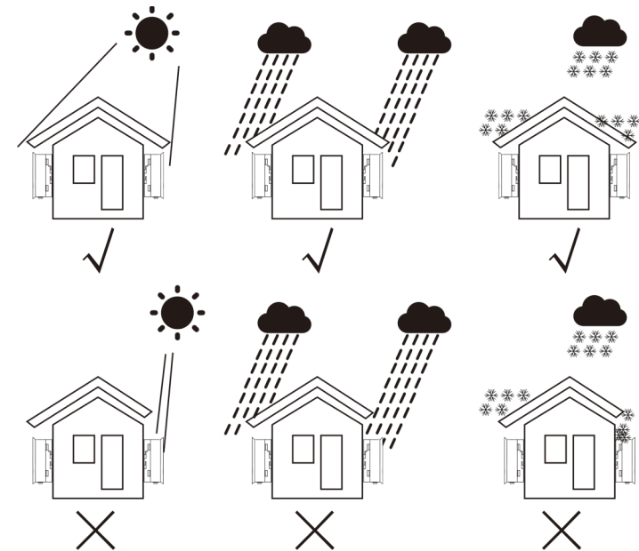
▲ Figure 5.1 Recommended installation position
