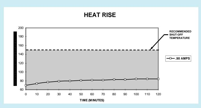
All of the pump models in the Performance Data and Heat Rise charts are in the shaded area, meaning they are capable of sustaining continual running, at any of the above listed pressures, without shutting down to allow the motor to cool. To conserve wearing parts, however, the pump should only operate as needed.
