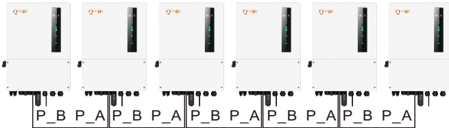
Figure 3.24 Parallel Terminal Connection
